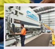
Sloanebuilt has an extensive range of inhouse equipment built to help keep you on the road. One of those is the 'Big Show'; an 1000 tonne 11m wide press which is able to bend bisalloy and hardox brands.
